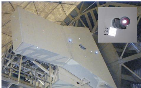
Figure 2: Reflective Tape Targets (2002) and Cat-Eye Reflectors (2008)
