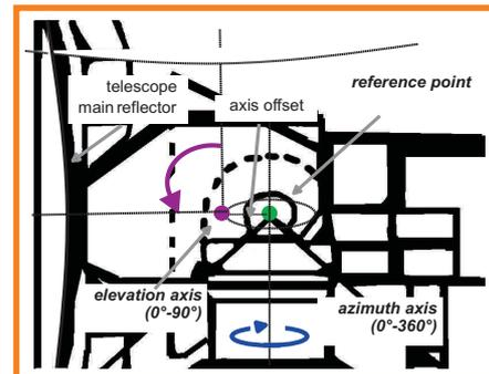
Figure 1: Definition of the IVS reference point
