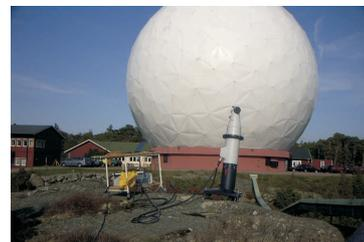
Figure 6: Laser Tracker in front of radome
